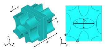
**Figure 2** Diagrams showing the parameters used to describe the systems modelled here. The parameter h indicates the thickness of the central block of material and is equal to d-2l.
