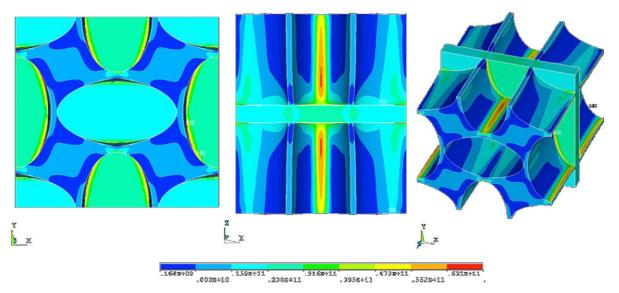
Figure 5 Diagram showing variations in stress intensity in a system which exhibits a Poisson's ratio of approximately zero.
