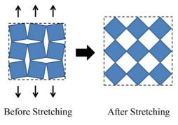
**Figure 1** A diagram showing the deformation of a rotating square system under the effect of tensile strain.
