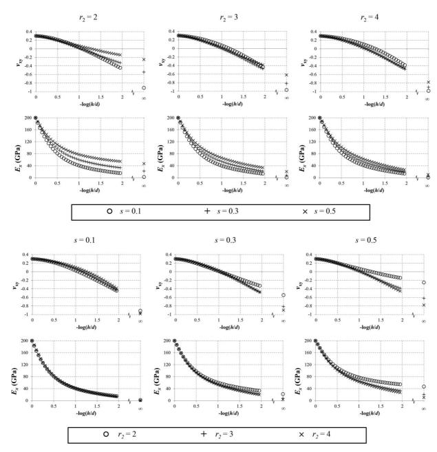
**Figure 3** Plots showing the variation of the Poisson's ratio and Young's modulus with increasing groove depth for systems with different s values, while keeping  $r_2$  constant (top panel) and with different  $r_2$  values while keeping s constant (bottom panel). Note that a value of 0 on the s-axis denotes a block of material without grooves while a value of s-corresponds a fully perforated system.
