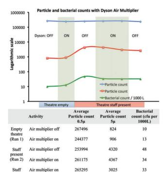
237314 Figure 1: Results of average particle counts (0.5 and 5  $\mu m$ ) and bacterial counts during a simulated operation with and without the Dyson Air Multiplier.
