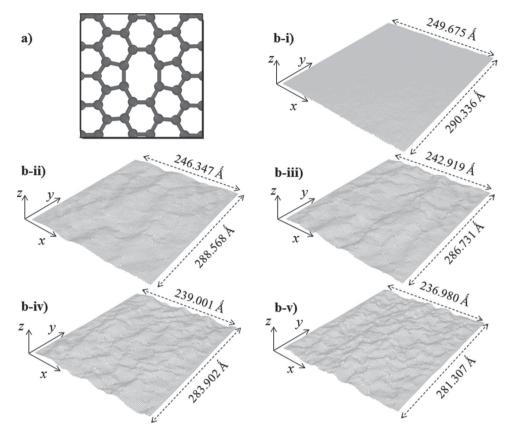
**Figure 1.** a) A representation of a 5–8–5 double vacancy defect in graphene and b) typical images of different systems at increasing defect concentration: i) p = 0.9%, ii) p = 0.5%, iii) p = 0.0%, iv) p = 2.0%, and v) p = 3.0%. Note that as the concentration of defects increases, the graphene sheets adopt a more wrinkled conformation thus achieving a shape which resembles that of a wrinkled paper model.
