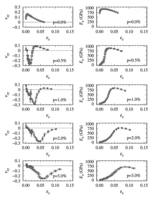
**Figure 3.** The averaged in-plane Poissons's ratios and Young's moduli (calculated from the differential strains) plotted against the engineering strain for stretching in the *x*-direction as obtained from the simulations of pristine graphene (p = 0.0%) and the imperfect graphene systems (p = 0.5%, 1.0%, 2.0%, and 3.0%).
