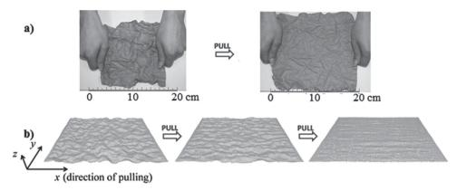
**Figure 2.** a) Typical images of a crumpled sheet of paper at different levels of applied strain and b) typical images of a graphene sheet having 3.0% defects at different levels of applied strain. Note that both systems undergo a de-wrinkling process so as to assume a more planar conformation resulting in an in-plane negative Poisson's ratio.
