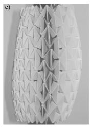
Fig. 9. Images of "tubes" formed from (a) a semi re-entrant honeycomb; (b) a conventional honeycomb and (c) a re-entrant auxetic honeycomb. Note that only the semi re-entrant honeycomb can be easily shaped into a tube since the conventional honeycomb tends to assume a "concave" shape whilst the auxetic honeycomb tends to assume a "convex" shape.
