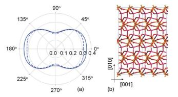
FIG. 3. (Color online) (a) The Poisson's ratios in the (010) plane (solid line,  $0^{\circ}$  corresponds to  $\nu_{[001][100]}$ ) and the (100) plane (broken line,  $0^{\circ}$  corresponds to  $\nu_{[001][010]}$ ) and (b) the structure of NAT in the (100) plane which is similar to that in the (010) plane.
