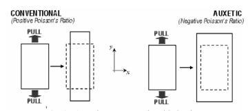
Fig. 1: Auxetic vs. conventional behaviour
