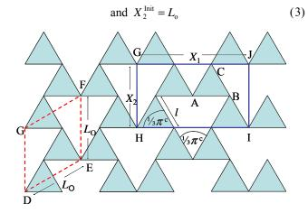
**Fig. 6:** The unit cell GHIJ used in the analytical model and its relationship with the 'minimal' unit cell DEFG
