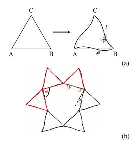
Fig. 7: (a) The changes in shape of the triangles due to loads; (b) the relationship between  $\omega$  and  $\phi$ .
