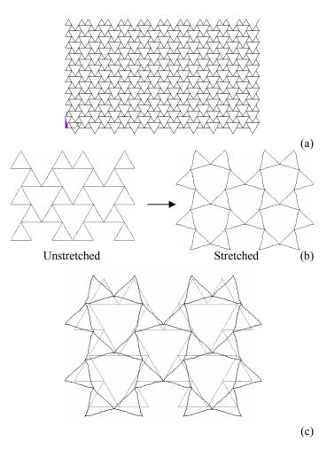
Fig. 5: (a) The 'unstretched' system constructed in ANSYS; (b) part of the system simulated in ANSYS in the 'unstretched' and 'stretched' (10% strain in the X-direction) form; and (c) a 'to-scale' superimposition of (b) to illustrate that the two systems have the same aspect ratios.
