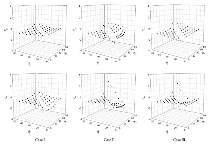
Figure 2 | Graphs showing the Poisson's ratios in  $v_{yz}$  and  $v_{zy}$  planes for hierarchical structures with different  $\theta_0$  values. The missing values for  $\theta_0 = \theta_1$  in both sets were due to unattainable geometries which resulted from mathematical constraints.
