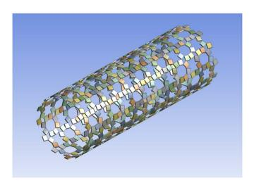
Figure  $4 \mid$  Stent based on a two level hierarchical rotating square geometry.
