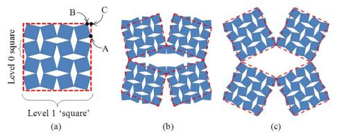
Figure  $3 \mid (a)$  Diagram showing the different points from which the Level 1 unit could be connected to other units (b) a two-level system with an acting rotating unit with a parallelogramic shape and (c) with a rectangular shape.
