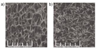
**Figure 5** The microstructure of the auxetic foam when immersed in a solvent where the foam was (a) unconstrained and (b) constrained in a rigid container of equal dimensions. The scale indicates a distance of 5 mm.
