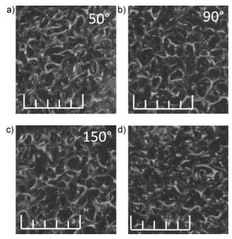
**Figure 4** The microstructure of the auxetic foam when subjected to (a)  $50\,^{\circ}$ C, (b)  $90\,^{\circ}$ C, (c)  $150\,^{\circ}$ C and (d) to the latter temperatures whilst the auxetic foam was in a rigid container of equal dimensions. The scale indicates a distance of 5 mm.
