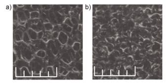
**Figure 2** The microstructure of (a) the original foam and (b) the auxetic foam. In both cases, the scale indicates a distance of 5 mm.
