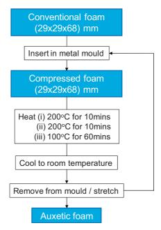
**Figure 1** (online colour at: www.pss-b.com) Summary of the thermo-mechanical process used to produce the auxetic foams in this work.
