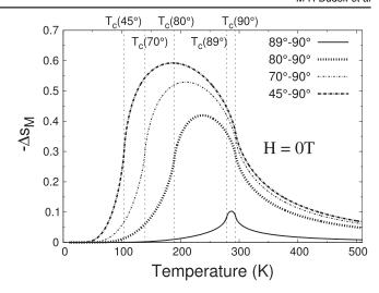
**Figure 2.** Temperature dependence of the isothermal entropy change  $\Delta s_M$  for MAS deformed from  $\theta_i$  to  $\theta_f$  at zero magnetic field. The plots representing deformations  $89^\circ \to 90^\circ$ ,  $80^\circ \to 90^\circ$ ,  $70^\circ \to 90^\circ$ ,  $45^\circ \to 90^\circ$  are shown (units in degrees). The vertical lines indicate location of  $T_c$  for a given value of  $\theta_i$  and  $\theta_f$ .
