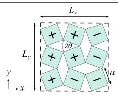
**Figure 1.** Magneto-auxetic system of  $3 \times 3$  squares of dimension  $a \times a$  with the exemplary configuration of Ising spins  $s = \pm 1$  denoted by '+' and '-' respectively, located at center of mass of the squares.  $L_x$  and  $L_y$  denote linear size of the system in the x and y directions respectively.
