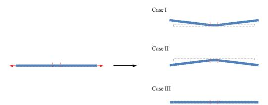
**Figure 7** The deformed and undeformed systems for cases I–III, the red dotted line highlight the region over which constraints where applied, on either the top/bottom nodes or both as discussed in text, where it is evident that uneven constraints are affecting the mode of deformation of the ligament.
