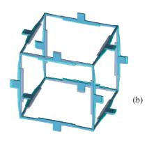
**Figure 12** (a) One of the possible models one may build using this simple concept, where, upon uniaxial loading in z one may observe (b) an expansion in x resulting in a negative Poisson's ratio,  $v_{zx}$ . One may also observe that the ligaments along z curve in both x and y which indicates that correct building of other systems may result in out-of-plane bending.
