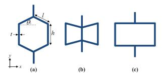
**Figure 1** Different possible configurations for centrosymmetric hexagonal honeycombs with (a) Y-shaped joints, (b) arrow shaped joints and (c) T-shaped joints.
