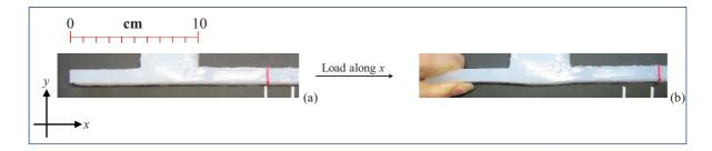
**Figure 6** The undeformed (a) and deformed (b) photos of a simplified physical model built from silicone material. On stretching along the length of the horizontal ligament, the response described above, where the shorter rectangular block extending from the top surface of the longer block is prohibiting this surface from deforming, is clearly evident.
