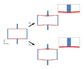
**Figure 4** The deformed and undeformed structure for a typical system for loading by a 5% tensile strain in x and y, suggesting that for loading in x, non-uniform deformations occur in the region of overlap of the vertical and horizontal ligaments, indicating that deformations other than simple stretching occur in this region, resulting in the observed curvature of the horizontal ligament at this point of overlap.
