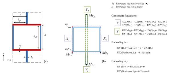
**Figure 3** (a) The unit cell chosen for simulating these systems. Note that as  $t \to 0$ ;  $l_{\text{eff}} \to l$ , and  $h_{\text{eff}} \to h$ , and the honeycomb reduces to the one shown by the solid black lines. The red rectangles indicate the horizontal ligaments, while the blue rectangles indicate the vertical ligaments. (b) The boundary conditions applied to the system to ensure tessellatability of the unit cell.
