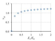
**Figure 8** Figure showing the relationship between the Poisson's ratio,  $v_{xy}$ , against the ratio of the Young's moduli,  $E_v/E_h$ , for a system having typical values of l = 10,  $h_{\rm eff} = 10$ ,  $t_1 = 0.2$ ,  $t_h = 1$ , where  $E_v$  is the Young's modulus of the vertical ligament and  $E_h$  is the Young's modulus of the horizontal ligament.
