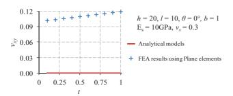
**Figure 2**  $v_{xy}$  as predicted by FEA simulations using plane elements and the analytical models of Masters and Evans [4], Gibson and Ashby [2], and Grima et al. [5], for different values of t, at  $\theta = 0^{\circ}$ . The analytical models predict a value of zero for any value of t, while the simulations predict a non-zero value, which appears to be dependent on the thickness of the ligaments.
