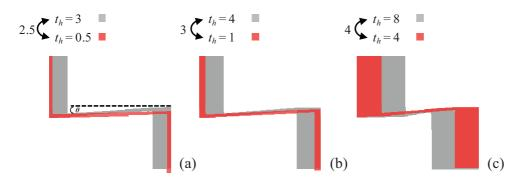
**Figure 9** Superimposed images of a quarter of the unit cell for systems with different values of  $t_h$  after a 0.1% strain was applied on the system, with a displacement scaling of ×40 of the original, showing that (a) at first for an increase in  $t_h$  there is an increase in  $\theta$ , then beyond a point (b), the increase becomes less pronounced and (c) the increase in  $\theta$  is not large enough to result in a system with a larger Poisson's ratio.
