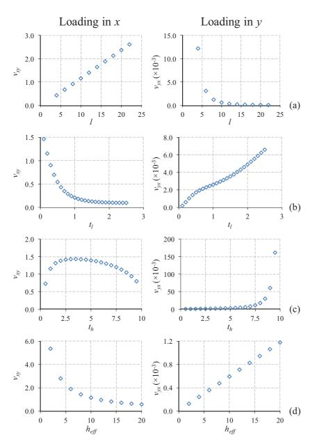
**Figure 5** The Poisson's ratio obtained from FEA simulations for the honeycomb systems at  $\theta = 0^{\circ}$ , for the system described in Fig. 3 having typical values of l = 10,  $h_{\rm eff} = 10$ ,  $t_1 = 0.2$ ,  $t_h = 1$ , apart for the varying parameter, where the changing parameter had values as described in the methodology for the respective graphs. Note the difference in scale for  $\nu_{xy}$  and  $\nu_{yx}$ .
